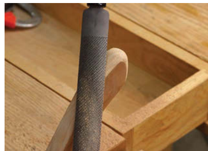
Rough start. A coarse rasp removes a lot of material in a hurry, but leaves a surface that looks rough.
