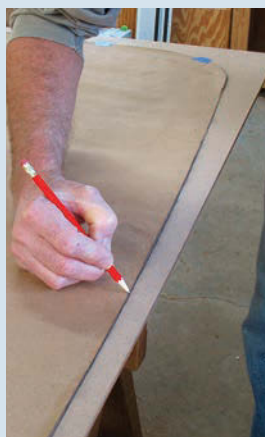
Paper transfer. Once satisfactory curved shapes are achieved on paper, the shape is traced on to MDF to create the template.
