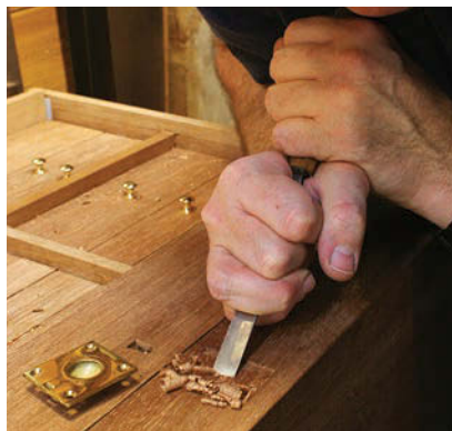
Moxon style. Using a paring technique described by Joseph Moxon, I carefully excavated to my knifed line. Once the cavity was roughed in, I smoothed it with my router.
