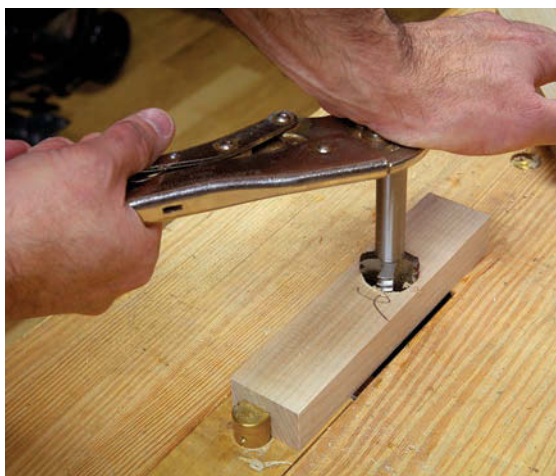
Tap the holes. A simple pair of locking pliers can help you turn the tap into the holes in the frame.
