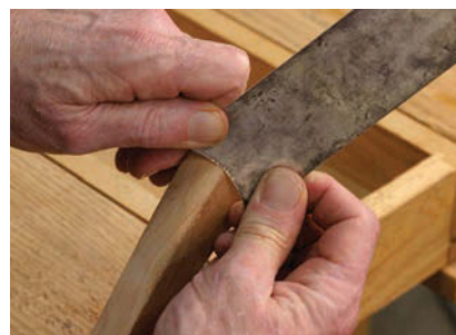
Easy scrape. A card scraper shaves off the high spots left by the finest-grain rasp. This is quick work because only the ridges left by the rasp need to be removed.
