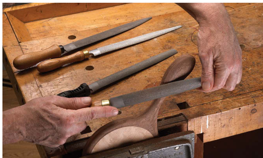
Quick & controlled. A good rasp makes quick work of shaping and refining curved surfaces.
