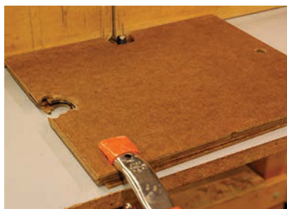
Shims step your cuts. Set your bit for its final depth of cut and use shims to surround it. Remove a shim after each cut to make the next cut deeper.
