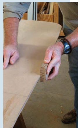
Fair is fair. Any irregularities on the template edge are sanded smooth to ensure a fair curve.
