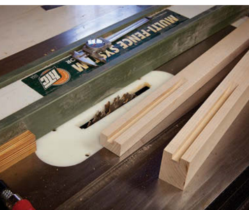
Essential grooves. Before you do any assembly, cut the grooves for the wagon vise.
