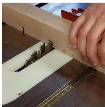
Digging for dogs. Cutting the dog holes using a dado stack makes for crisp work.
