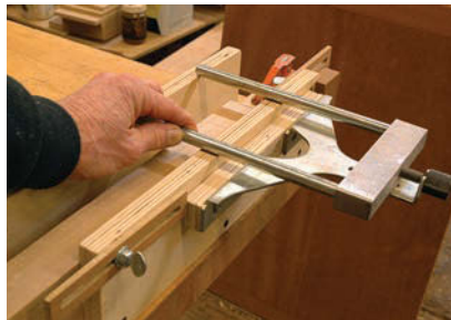
Three stops. A fixed stop attaches at one end with an adjustable stop at the other end. An adjustable stop on the inside of your jig registers your workpiece.
