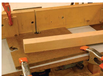
Stop it. To set the length of your mortise, clamp stops to the fence. Start with the workpiece tight to the right stop and plunge down onto the bit. Once you are at depth, move across the bit to the left stop.
