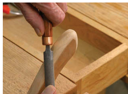
Getting close. The surface begins to develop a sheen as an even finer rasp removes the marks from the previous tool.
