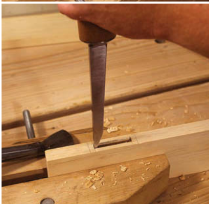
Chopping a mortise. I chop a V-shaped chip from the center of the mortise until the center is at full depth. The last two chops are right at the knife lines to define the ends of the mortise.
