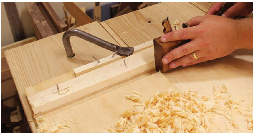
Riding the fence. Plane the dado across both case sides at the same time to guarantee that the dados line up in the assembled case. Leave the nails in the fence and battens proud for easy removal.
