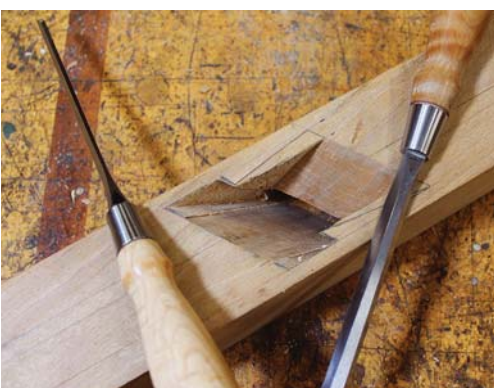
Bed as reference. To fair the bed to the abutments, place a paring chisel flat on the bed at an angle and skew cut into the abutments.
