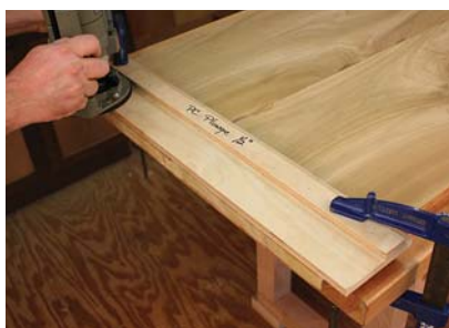
Edge-routing jig. Used for trimming boards to length, cutting dados in case sides and tenons on tabletops, this jig makes routing accurate and safe.
