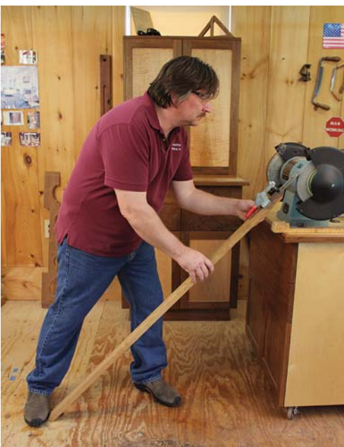
Plane iron sharpening jig. Used to hollow grind a plane or spokeshave iron, this jig makes grinding fast and repeatable.
