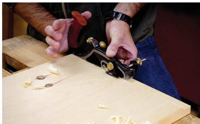
Squaring rabbets. Cross-grain rabbets help square the carcass and line up the pieces during assembly.
