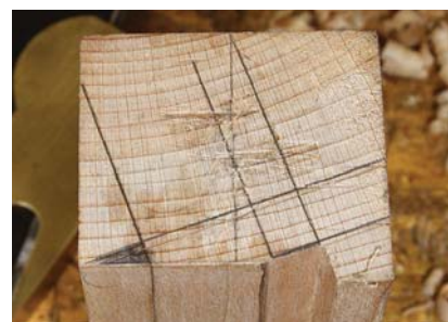
Double-check. There should be a gentle arris between the bevel face and the tongue face. Pencil the line to verify that it's straight and parallel along the length of the sole.
