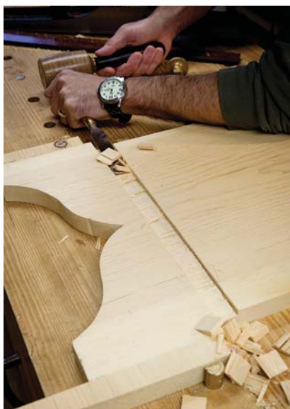
The hungry chisel. A chisel takes a bigger bite than a router plane, so do as much work as possible with the chisel.
