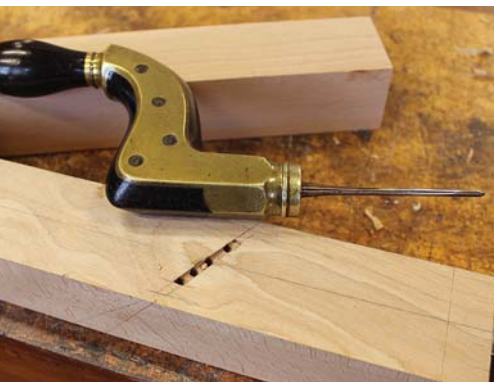
Don't open wide. The mouth must be tight, so drill within the lines. I use a brace and shell bit because a shell is simple to adjust within the cut as needed.
