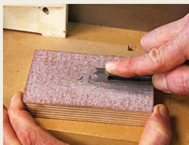
Don't overdo it. Chisels will benefit from removing grinding marks and a light honing. Polishing them to a perfect edge is a waste of time.
