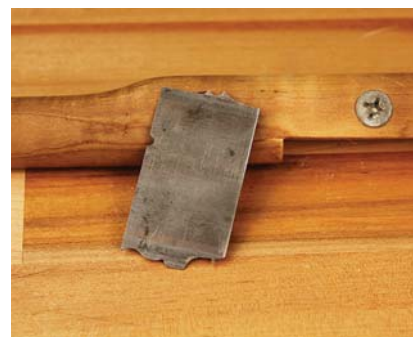
Scraper shapes. The most common moulding created with a bader is a bead, but other profiles can easily be created as well.
