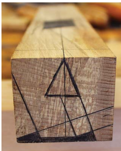
Laid out. The five spring lines are what guides the remaining work. You can also see the midline and how the spring lines relate.
