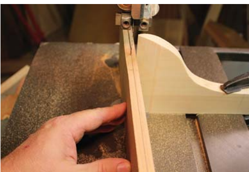
Single-point resaw fence. A single-point fence for your band saw is a simple, quick-to-make jig that provides all the resawing accuracy you need.
