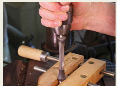
Alignment only. The sharpening cone can be placed in the drill press to keep it in line with the chisel. A few twists by hand are all it takes to hone the inner surfaces.
