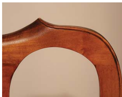
Bead the edge. On Queen Anne dining chairs the rear legs and crest were often beaded. This decorative treatment could not be accomplished with moulding planes.
