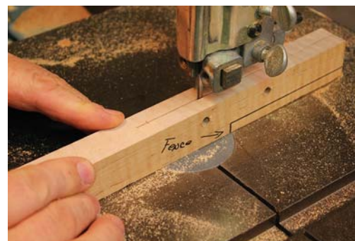
Cut the bader. Saw a kerf through the end of the bader that will hold the cutter. Make sure it passes both bolt holes to ensure adequate clamping pressure.
