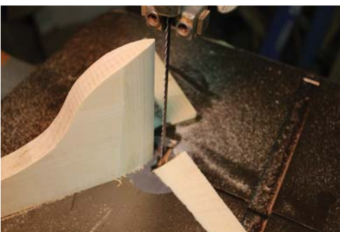
Get to the point. On the band saw, shape the leading edge of the stock to a point. I like to leave it blunt with a flat of about \frac{1}{16} " wide.
