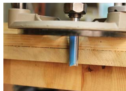
Depth of cut. In order to determine how thick the base of the jig can be, place your router on the base then measure to ensure the bit reaches through the cut.
