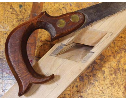
Tight quarters. The small opening in the mouth requires a small saw. This is where the keyhole saw shines.
