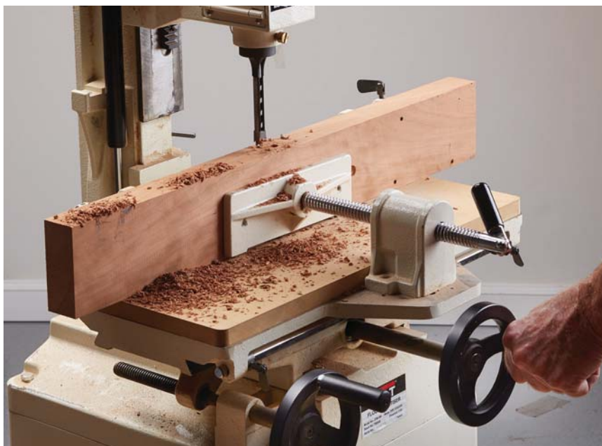
Big difference. The sliding table on floor-model machines dramatically increases efficiency over benchtop models.
