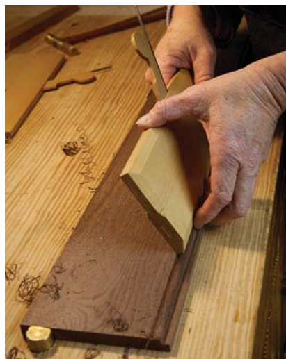
Moulding planes. The rabbets and grooves will help to guide the moulding planes as you shape the profile. A light touch is key when using these traditional tools.
