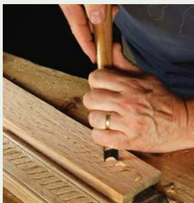
Hand power. You do not always need a mallet when carving. Here my two hands work together to guide my chisel.
