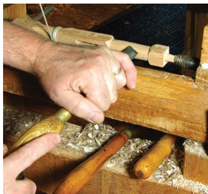
Simple lathe work. Tenons for the ratchet arms are cut, then the rounding begins. Your skew may become your best friend.
