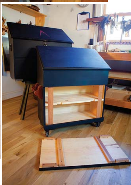
Large or small. To safeguard your tools, both versions of the Dutch tool chest feature fall-fronts with a resourceful and simple locking mechanism.
