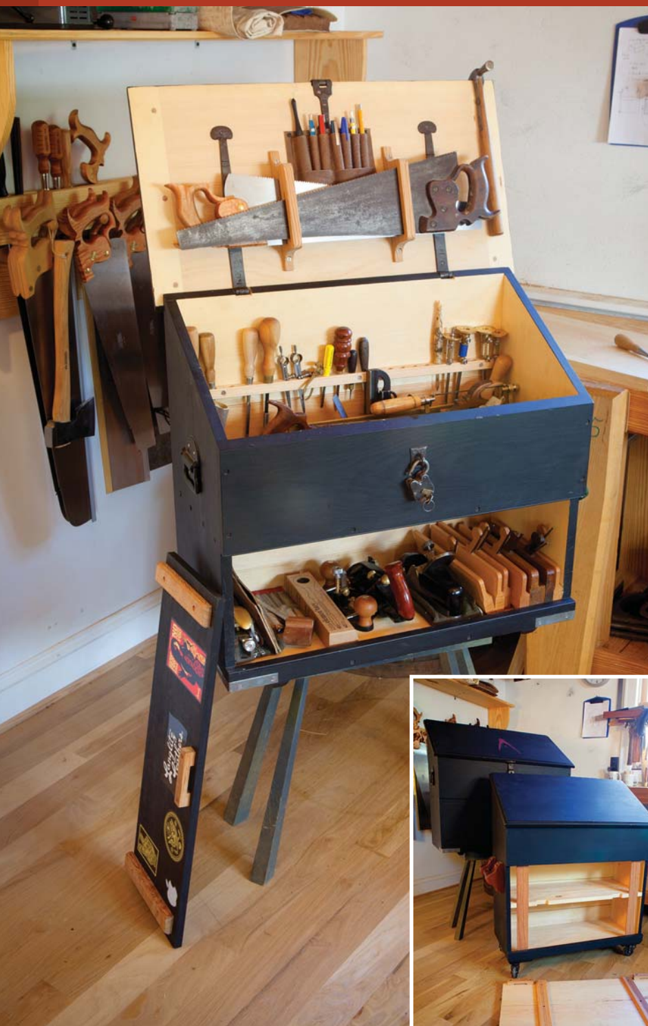
Large or small. To safeguard your tools, both versions of the Dutch tool chest feature fall-fronts with a resourceful and simple locking mechanism.
