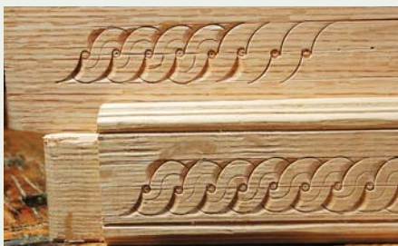
That's nice. The carving work on the top rail looks great when completed. A few gouge cuts results in a lot of detail.
