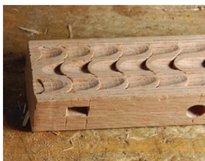
Mortise types. The mortises for the shelf and crosspieces are bored. For the shelf, work is completed using a paring chisel.
