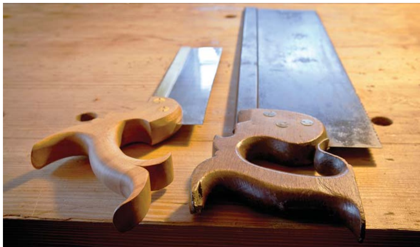
Two very different hang angles. All of the variables in motion make each type of saw something of a separate art.
