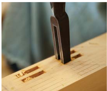
Two mortises, one chisel. A double-bladed chisel is used to chop the paired mortises in the stiles.
