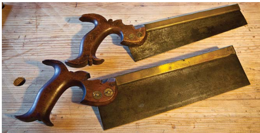
Blade rake. This is one reason that numbers don't matter. These saws have the same numerical hang angle, but they won't feel identical in use. The saw with the raked blade is more compact.
