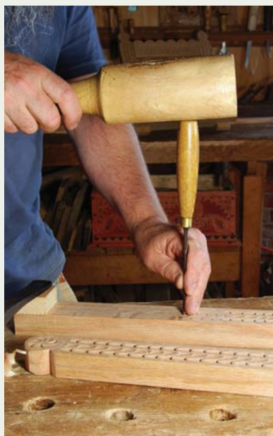
An alternate posture. Grip the tool near the cutting edge with your fingers on the back of the gouge and thumb on the front. With this grip, rest your fingertips on the board you're carving to steady the gouge.
