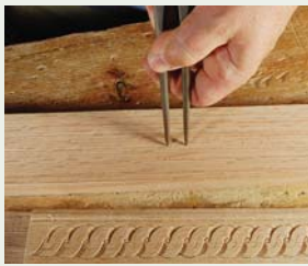
Step-off marking. A compass makes quick work when laying out the braid design.
