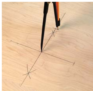
Connect the dots. Set the compass between the center and the end of the line, then swing an arc to cross the vertical line. Connect those points to make a 45° angle.
