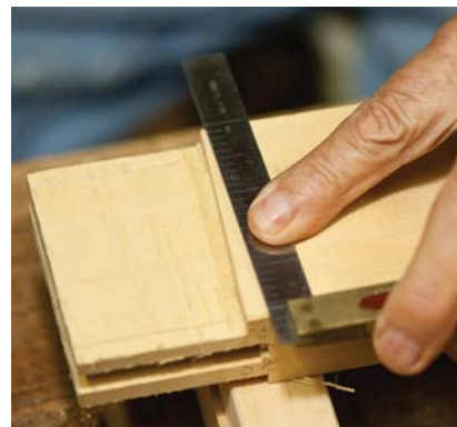
Not square. The shoulder of the dividing rail is angled to match the bead below with the bevel above.
