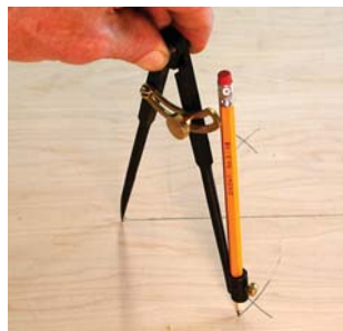
Above & below. Swing arcs above and below a line from both ends so they intersect. Connect those points to divide the line squarely into two equal segments.
