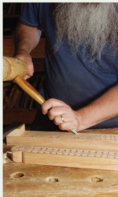
Dig a little deeper. As you drive forward, the gouge cuts deeper until it comes right up to the incised cut to pop out its chip. Voilà!
