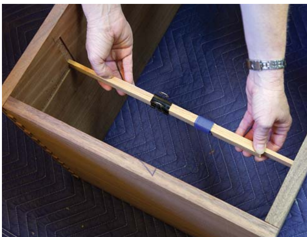
Pinch sticks. My usual pinch sticks are too long to fit across the chest's depth, so I cobbled together a set with two offcuts, a binder clip and some blue tape, sticky side out (then wrapped with a piece of tape sticky side in to keep things nice and neat).
