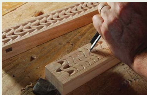
Making waves. Chips behind the grooves are easily removed. Make sure you have the gouge pointed in the right direction to keep the wave flowing.
