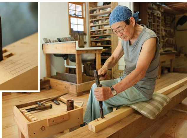
Two mortises, one chisel. A double-bladed chisel is used to chop the paired mortises in the stiles.
