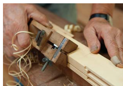
On the bevel. The stiles are beveled above the dividing rail.
