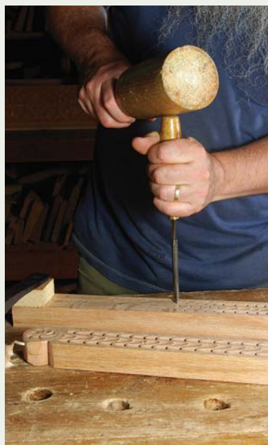
A handle grip. Hold the tool near the bottom end of the handle and brace your forearms against your torso to steady the gouge as you strike it with the mallet.
