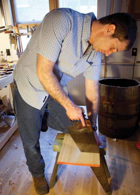
Sweet spot. The correct cutting trajectory is the perfect balance of forward and downward pressure.
