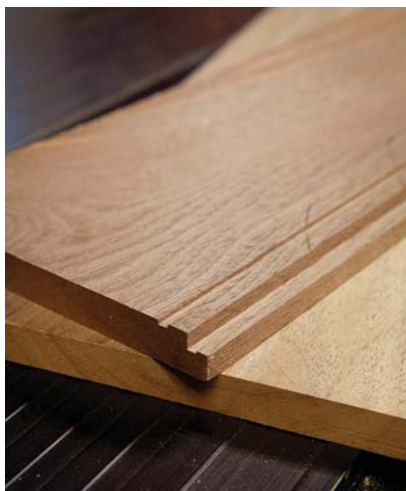
Rabbit first. Save yourself a lot of time (and get better results) by cutting rabbets and grooves to remove as much waste as possible before using hollows and rounds to shape a moulding profile. I cut these at the table saw.
