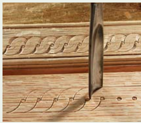
Braid beginning. The width of your gouge determines the amount of slope in your braid.
