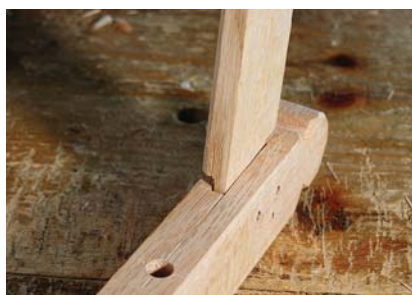
Flush at the front. With thinner stock, a bare-faced tenon allows for thicker mortise walls and tenons, and the face of the workpiece can be flush at the front.
