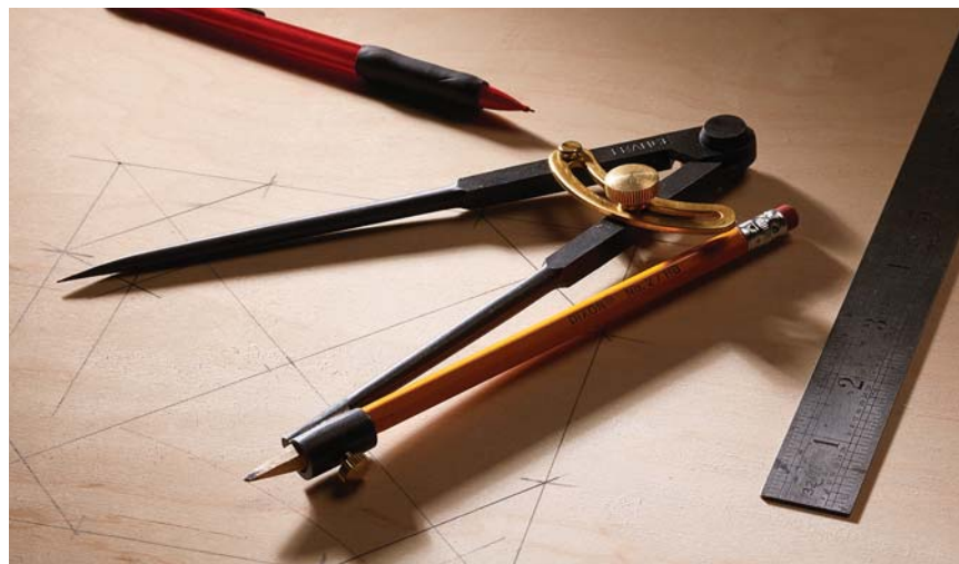
All shapes & sizes. With a compass, straightedge and pencil, you have a woodworking trifecta with which you can draw many geometric shapes.
