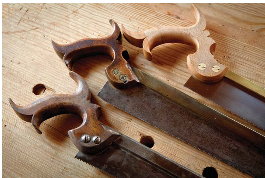
Fundamental character. Blade rake is like hang angle – there is no single correct value for it. A saw maker's decisions become a saw's fundamental character. All three of these saws are quite nice, and each is a little different.
