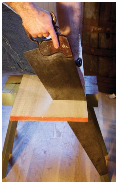
High & low. Notice the difference between these two hang angles. The one on the right has a hang angle that is far too shallow; it directs your energy up away from the saw's teeth. I suspect that is why this vintage saw is in such good condition – nobody liked using it.
