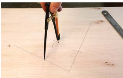
Divide & conquer. Swing arcs from the vertex of an angle, then make intersecting arcs from those points.
