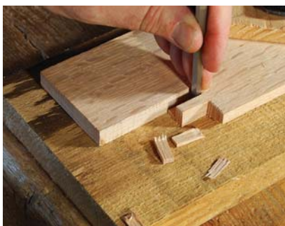
Detailed joinery. To get the shelf to slide past the front of the stiles, a little extra work is required. It looks complicated, but it's not.
