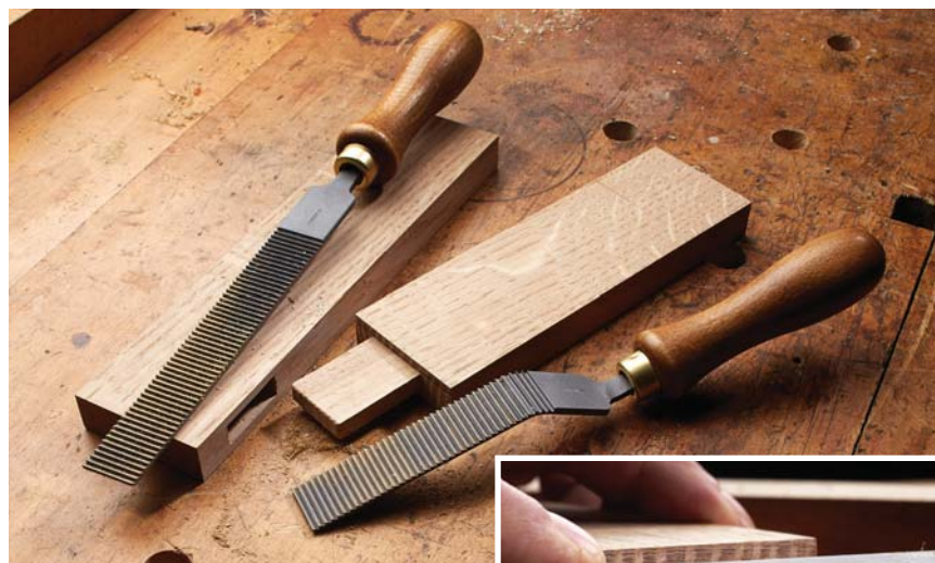
All in a row. A good float functions much like a wide saw or a gang of scrapers. It's an easy way to remove small amounts of material in a controlled and precise manner.
