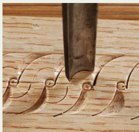
Find your center. Additional detail is added by using a smaller gouge to create lines that are centered between the earlier cuts.
