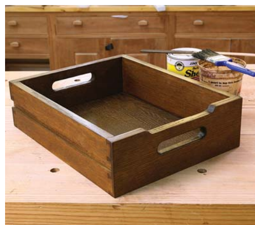
Drawers or Trays? Handle cutouts on the fronts and back, and a plywood bottom fully captured in grooves on all four sides, allow the drawers to be pulled out to function as trays – so finish all show surfaces.
