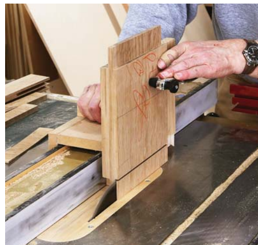
Tenon jig. A jig with a toggle clamp holds workpieces securely on end to safely cut tenon cheeks at the table saw.
