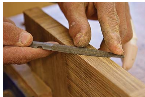
Finishing touch. After trimming, a detail file cleans up and softens the edges.
