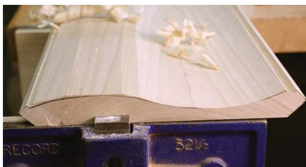
Faceted flats. To get to round, start by beveling the waste then knock those corners off to create more flats. Eventually you'll have so many facets it'll be easy to make it round. I use a block plane for this operation.
