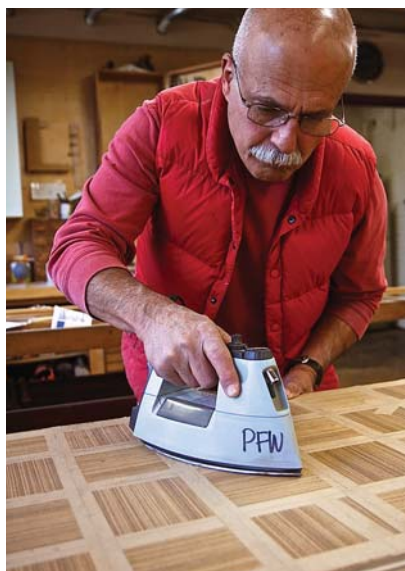
Bench press. The iron heats the veneer and the glue, adhering it to the substrate.
