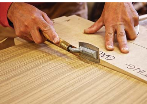
This way. The reconstituted veneer sheet is cut across the grain into 5"-wide strips.
