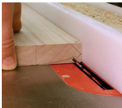
Rabbet it. To make large convex shapes, start by defining the outermost points of the curve with rabbets. They will act as guides for your handplanes.
