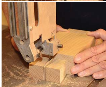
Machine-assist. For dovetails of this size, I cut my pins on the table saw and tails on the band saw, then clean up to the baseline with chisels.
