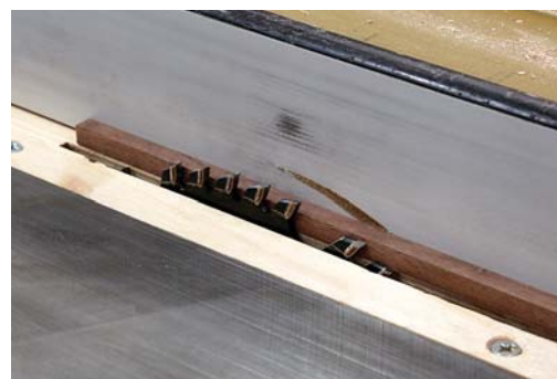
Trapped. Wood caught between the fence and the rising teeth of the blade is likely to be thrown back toward the saw operator.
