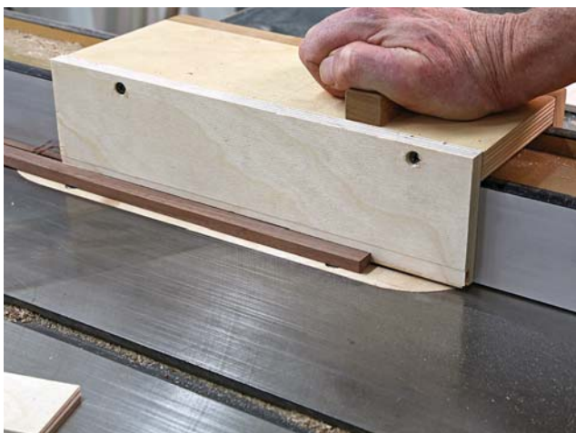
Ride the fence. A pusher that straddles the fence (along with a zero-clearance insert) makes it possible to rip thin pieces safely.
