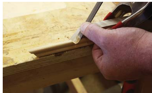
Slick trick. Use a scrap cut at a 45° angle to help guide the chisel as you pare the pointed cutout for the intersection of the double-arch moulding.
