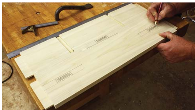
Accurate layout. On the back, each of the mortises are centered in the drawer openings and are set flush with the front apron. If these aren't correct, drawer problems are sure to arise.
