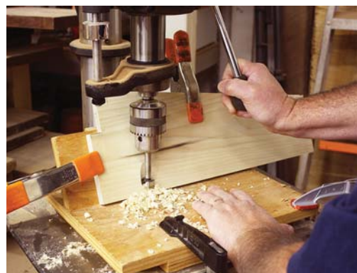
Laid back. The key to good pocket-screw holes using a press is to tilt the workpiece at 22 1/2° as you drill.
