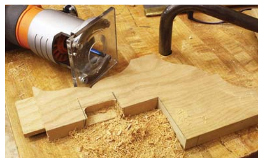
Exacting fit. Router waste removal produces a dead-flat socket front for the runner dovetail. A tight fit keeps the joint clean.
