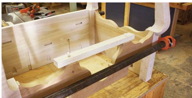
Stress relief. Use the finial holes to hold a temporary support in place as you clamp the lowboy front; this keeps the apron from cracking under stress.
