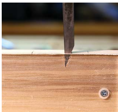
Size does matter. The mass of a mortise chisel enables it to drive deeper and remove more wood than a standard chisel.
