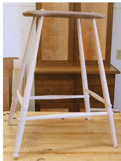
Dry-fit. Rough assemble the stool and trim the tenons close so the wedge placement can be marked.
