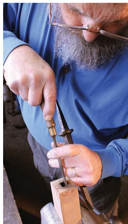
And test. With the hole burned out, I test the fit of the chisel tang.
