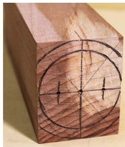
Centerpoints. Lay out one true center and two offset centerpoints on each end of the handle billet.
