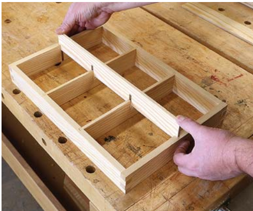
Easy does it. Your egg-crate joints should slip together easily with finger pressure only (and glue is overkill).
