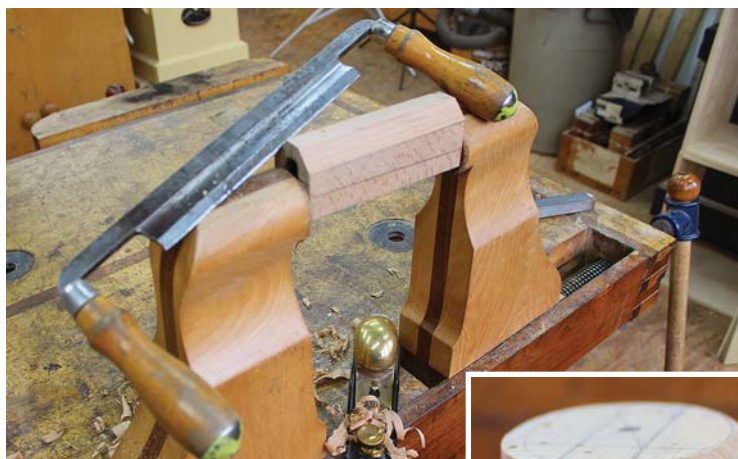
Shaping setup. My clamp for this sort of work resembles a lathe's headstock and tailstock. It holds the work securely as I shape the oval handle with a drawknife, block plane and spokeshave.
