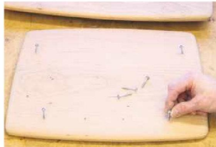
18 Remove the top for finishing and fit four screws as shown to act as temporary supports
