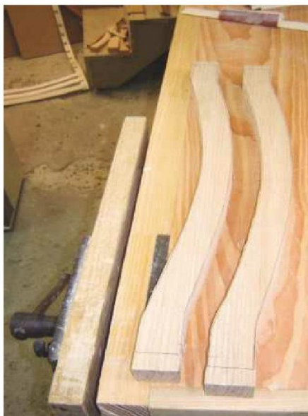
20 These solid curved elm rails are fitted at the top and tail of the seat frames
