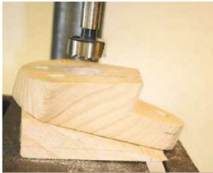
8 Finally, use a 25mm saw-tooth Forstner bit to drill the holes for the legs
