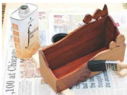
19 After final sanding brush on two coats of Chestnut Finishing Oil. Denib and complete with wax polish
