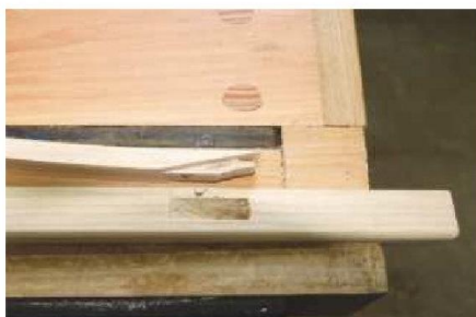
18 Cutting the other mortises to match the rib tenons was a case of trial and error...
