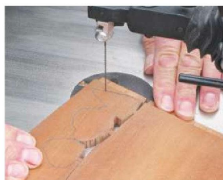
9 Drill holes for inserting blade where necessary. Follow the pencil line carefully on the scroll saw
