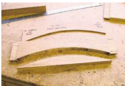
18 To speed up the repeat cutting, I made a rod for each chair rail pattern
