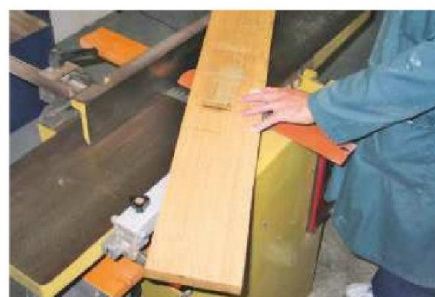
3 Any 'misses' that occur during surfacing can be removed during the thickening stage
