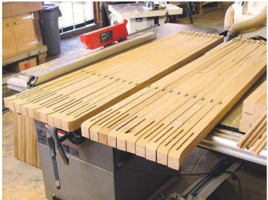
12 Then all the back legs were mortised ready to accept the chair rails
