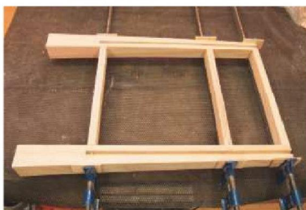
15 Glue and cramp up each pedestal front by assembling two legs and three rails
