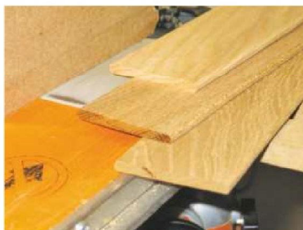
17 Machine both edges of an offcut to make the beading, then cut it to width
