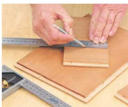
5 Carefully mark out positions of grooves for the divider panel on both end pieces
