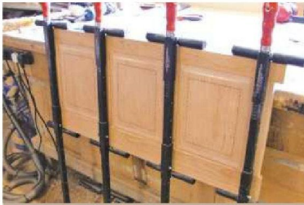
18 The panelled frame for the rear of the upper section is assembled and cramped
