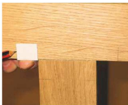
11 Dry-assemble the chest and mark the points where the frame chamfers will start and finish
