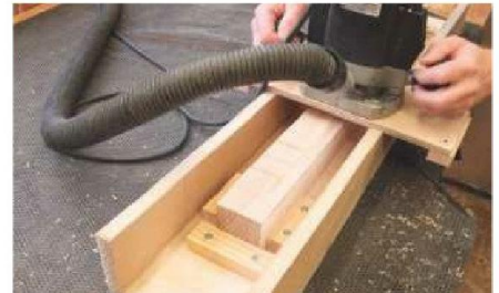
12 Shape each leg by making a series of shallow cuts with the router
