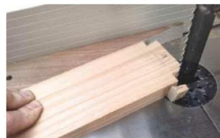
5 Cut the rail dovetails on the bandsaw against a 1:5 wedge held against the fence
