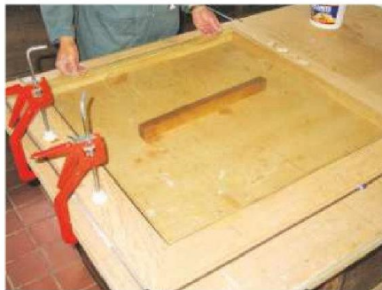
14 Mitre the corners, dry-assemble the frame and check that the glass fits in its rebate
