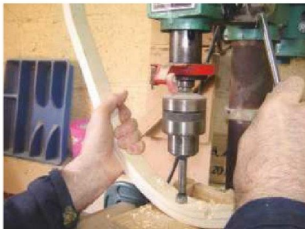
8 Use a Forstner bit in a drill press to remove most of the waste from the dovetail sockets
