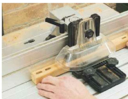
4 Round over the long edges of the legs using an ovolo cutter in the router table
