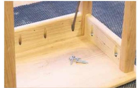
16 Align each frame on its tabletop and drive in the pocket hole screws to attach it
