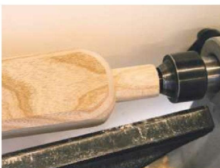
10 Turn the stub to a spigot and create a rounded chamfer on the leg as shown
