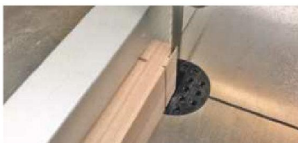
17 Cut the tenon cheeks on the bandsaw; take care not to overshoot
