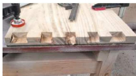
10 ...and remove the rest of the waste from the sockets with a really sharp chisel
