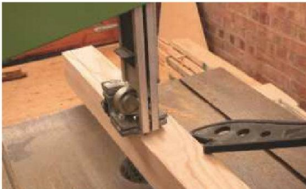
10 To save router time and cutter wear, rough-cut each leg to shape first
