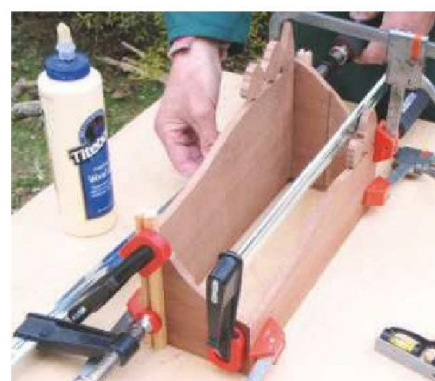
12 Cramp the box together on a flat surface. Check for square, adjusting cramps if necessary
