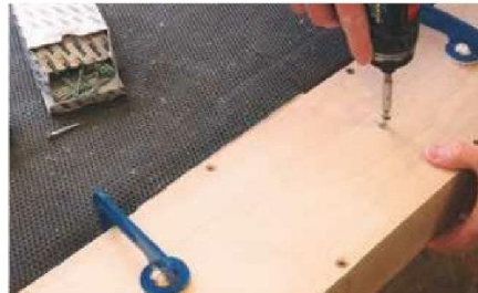
11 Cramp the rough-cut leg in the jig and secure it with two screws
