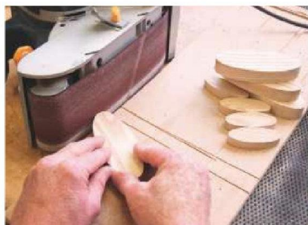
36 Cut four handles and four spacers and sand their edges smooth
