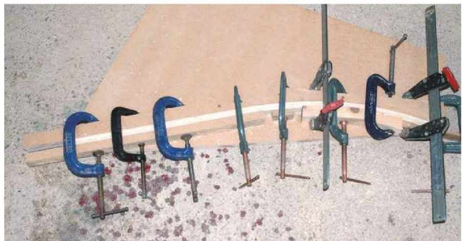
14 Make up the curved ribs as before by bending ash strips against a former
