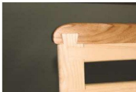
25 Attach the elm rails to the end-most slats with a dovetail, plus biscuits for extra strength
