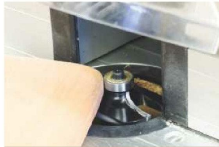
15 Remove the templates and round over both edges of each tabletop
