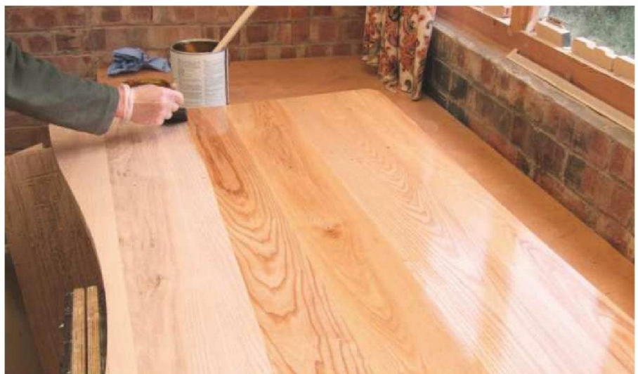
48 Apply hardwax oil and then liquid wax to the various components
