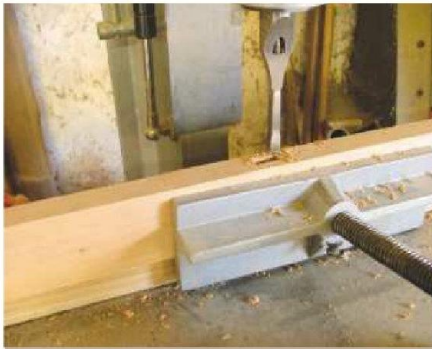
1 Cut all the mortises after machining the various frame components to size
