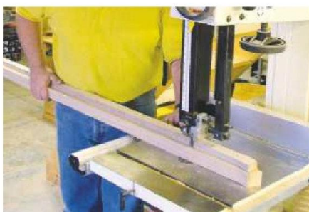
3 After screwing the rod to each blank, I removed the excess timber on the bandsaw
