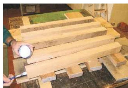
2 Prepare the rough-sawn components, then seal all the ends to prevent splitting
