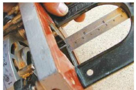
8 ...and then transfer the measurement to set the correct router cutter depth
