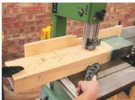
2 Cut out the eight leg blanks, then rip them to width on the bandsaw
