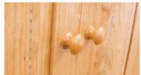
23 I turned a set of eight matching knobs and dowel-jointed them to the cabinet doors
