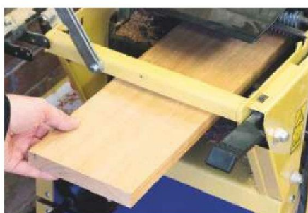
9 Thickness to 20mm the cherry boards that will make up the three tabletops
