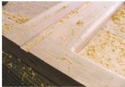
19 Cut a housing across the centre of the top and bottom frames to accept the central divider
