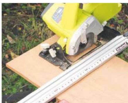
1 Thickness the timber to about 8mm and saw panels to length. Cut the front and back 2mm oversize
