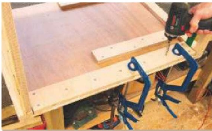
18 Add a strengthening batten to the inner face of each side panel, aligned with its top edge
