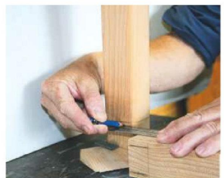
17 Use a pencil, block and straightedge to scribe each splayed leg, then cut it to length
