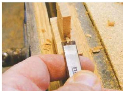
13 Clean up the shoulders on the tenons carefully with a sharp chisel
