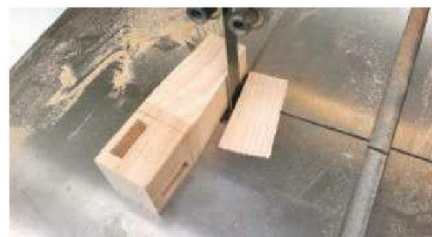
18 After a dry assembly of the frame, you can remove the legs and cut the tapers on them
