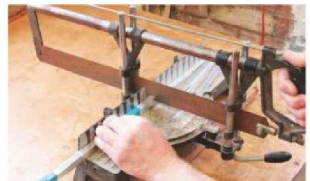
47 Cut the aluminium hanger rails to length with a fine-toothed saw and file their ends smooth
