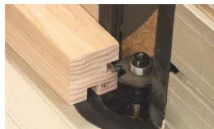
14 Cut the grooves to take the panels in the legs with a suitable cutter on the router table
