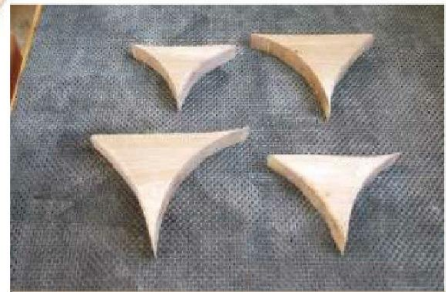
12 Cut the brackets out on the bandsaw; they're all slightly different sizes!
