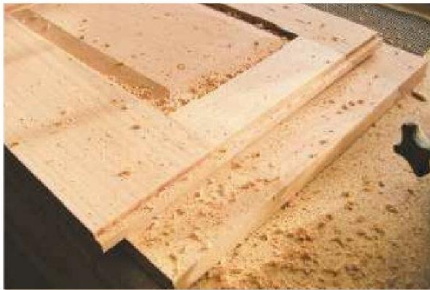
2 The inner panels contain one fielded panel and have a rebate along the bottom edge
