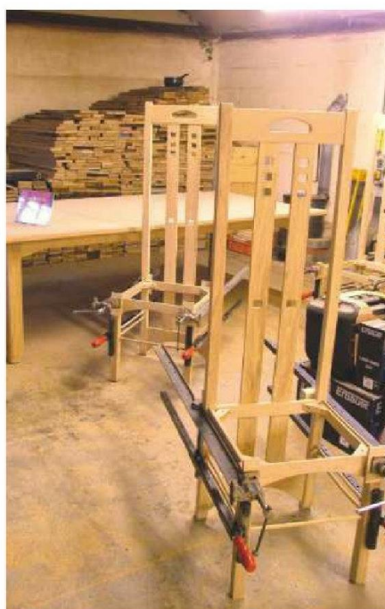
25 The front and back frames were married up by fitting the six side rails
