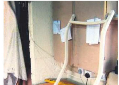
7 Cut the slats to length and store them together in a clamp until they're needed
