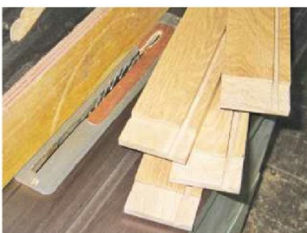
8 Machine a groove on the inner face of each rail to receive the top buttons
