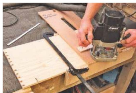
25 Rout two slots in the top of each filing drawer side to take the hanger rails
