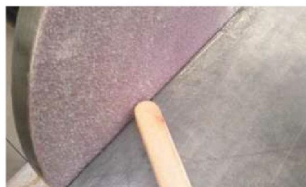
30 Cut the cleats to size and then round their ends on the disc sander
