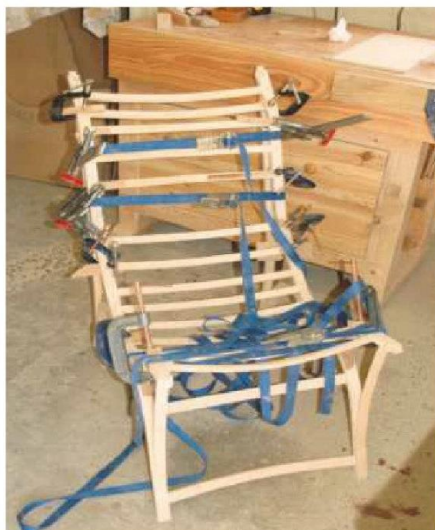
24 Glue the slats and cross-rails into their dovetails and cramp up the assembly as tightly as possible
