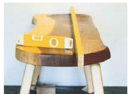
16 Stand the table on a flat surface and pack under its feet to get it level
