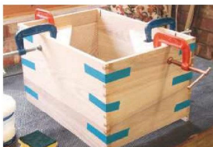
28 Tape and right-angled corner webs help to hold the assembly square
