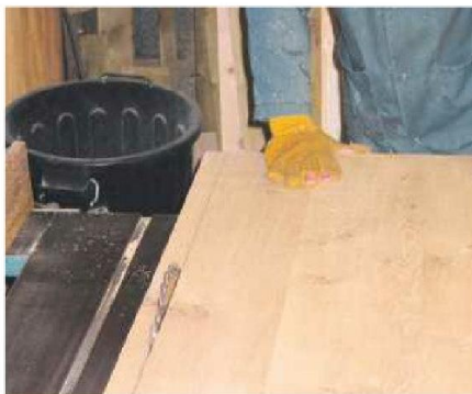
20 Cut the top to width on the bench saw and square the edges. The guard has been removed for clarity.
