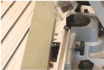
7 Use the template to cut each jig side in turn on the router table
