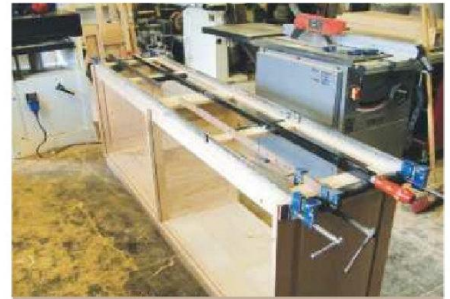
23 Assemble the base panel, the top frame, the end panels and the central divider
