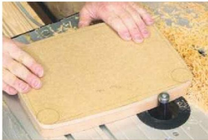
14 Cut each tabletop accurately to size on the router table using a bearing-guided straight cutter
