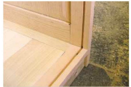
20 Form a groove in the end frames and the base panel to take the plywood back
