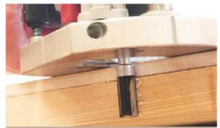
44 Reattach the template and trim the desktop precisely to size with a straight router cutter
