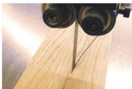
17 Use the bandsaw again to cut the curves into the front and rear rails
