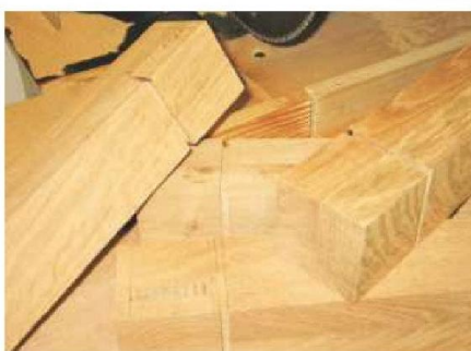
5 Cut a groove on the two outside faces of each leg to accept the decorative beading later
