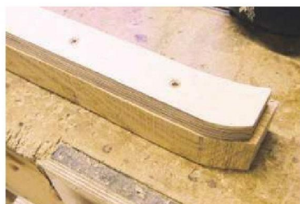
4 This left a couple of millimetres all round for cleaning up on the spindle moulder
