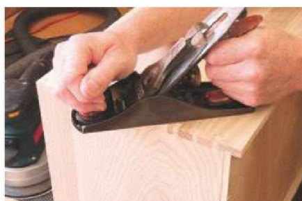
30 Use a sharp hand plane to trim the protruding pins and tails flush
