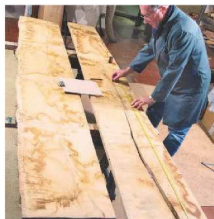
1 When marking out the various components, take care to avoid knots and splits
