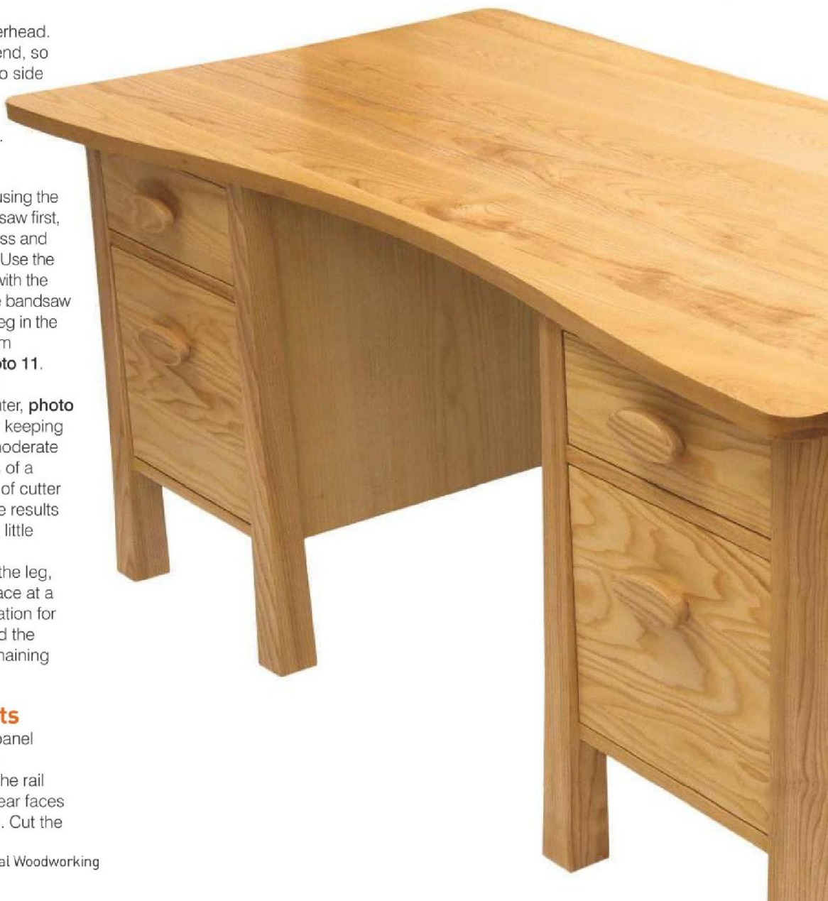
16 Assemble two rear legs and a back panel, then add in the two side panels
