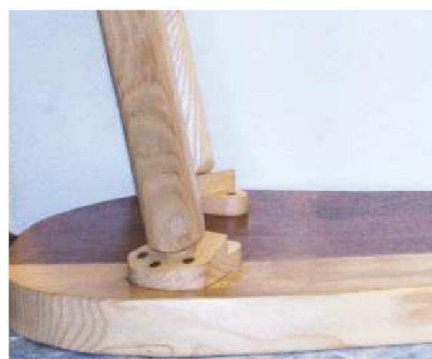
15 Apply glue to each spigot and twist it slightly as you push it into place to spread the glue
