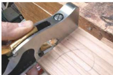
24 Trim the tenons with a shoulder plane if necessary to get a good fit
