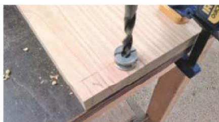
9 Drill out the waste between the dovetail pins using a twist drill fitted with a depth stop...
