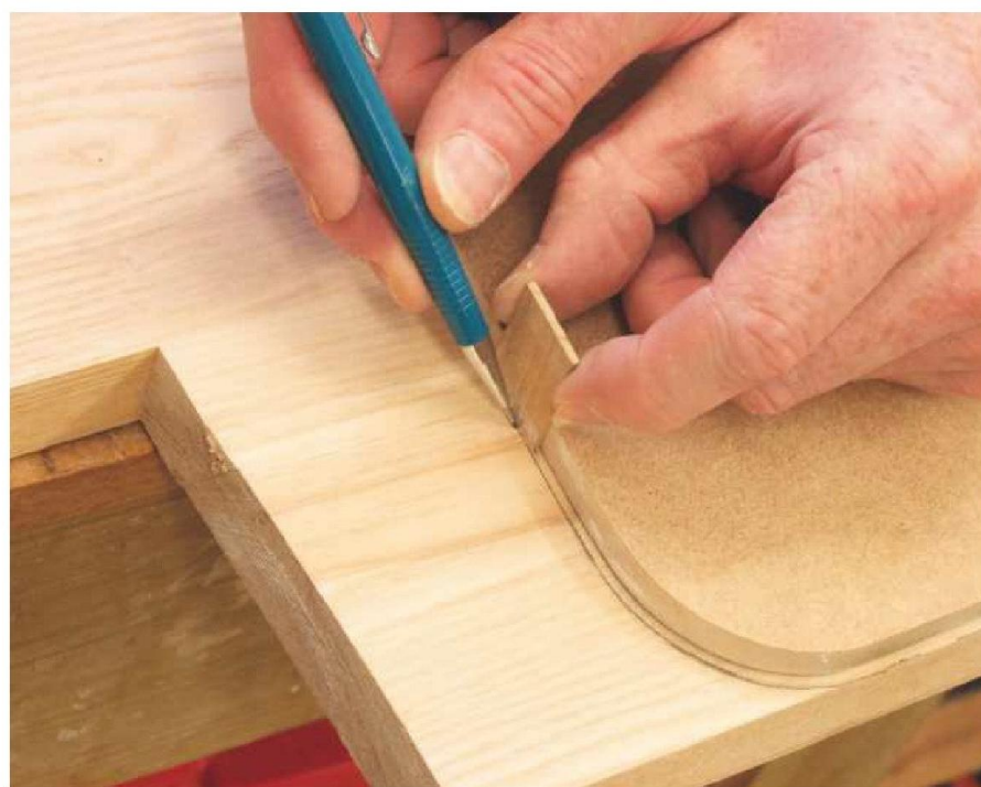
42 Draw around the template with a slim spacer to mark up the desktop
