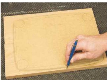
12 Mark each tabletop profile on its panel using the appropriate template
