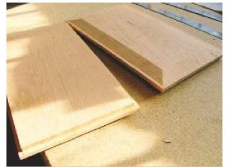
11 Form a rebate on the back of each panel to create a tongue all round
