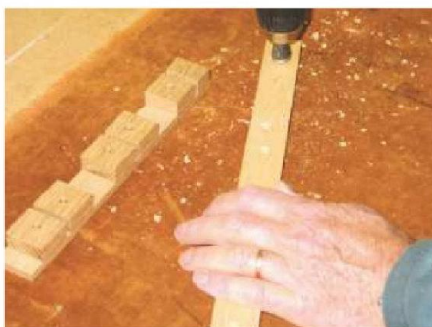
16 Shape and drill the buttons in a strip before cutting them off to length
