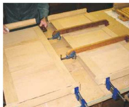
13 Cut the panels to size, then assemble the front and the back sections
