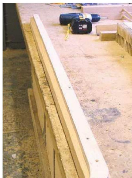
2 A 12mm-thick plywood rod guaranteed that all the back legs would be identical
