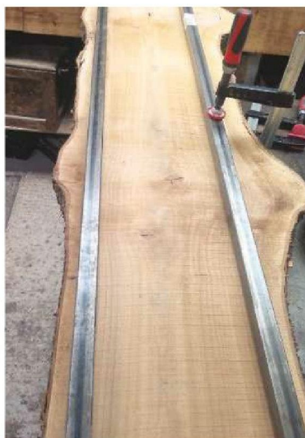
2 Mark parallel edge lines on each board and saw off the sapwood
