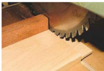
15 I used my radial arm saw to remove the waste from the tenon cheeks...
