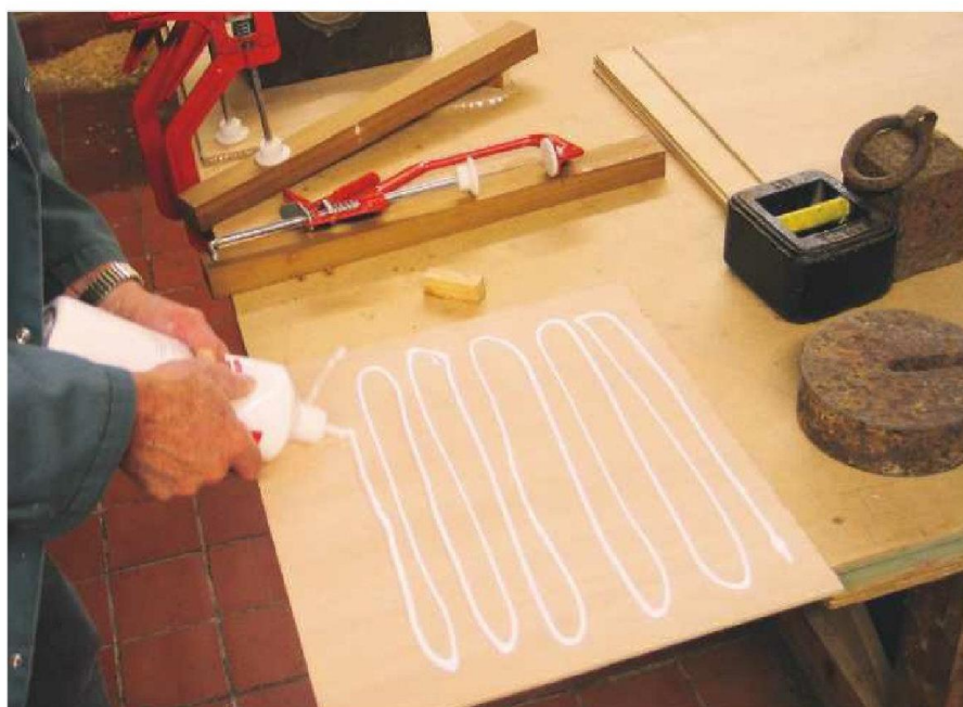
10 Prepare the panels by gluing one surface and rubbing the other onto it
