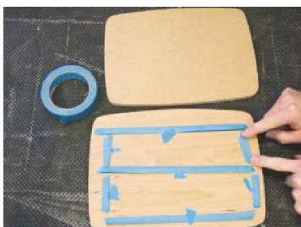
13 Attach each template securely to its panel with double-sided adhesive tape
