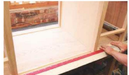
45 Place the desktop face down and carefully align the two pedestals on it
