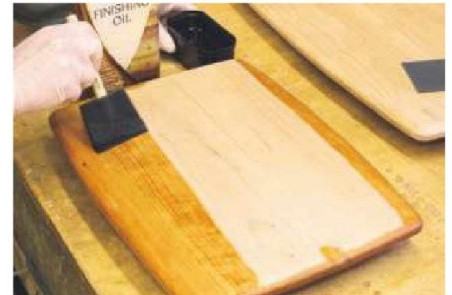
19 Apply finishing oil with a foam brush, sanding down lightly between coats. Then wax it
