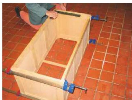
14 Complete the chest carcass by fitting the end rails and panels in place
