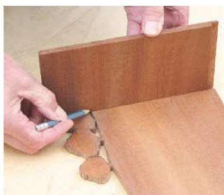
10 With the outlines cut on front and back panels, mark the height on both end sections
