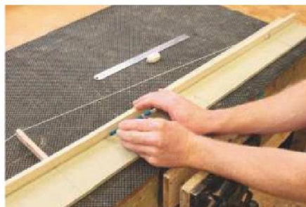
4 Use the bow and string method to mark the arc on the MDF template
