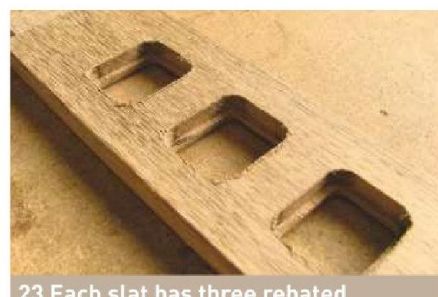
23 Each slat has three rebated apertures cut out for a stained glass insert. They need squaring up...
