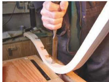
9 Then cut each socket accurately to size with a sharp chisel and a mallet
