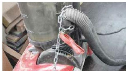
13 Earth your extractor to eliminate the risk of static electric shock from the fine dust
