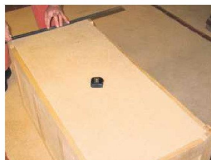
16 Mark the dimensions of the base panel from underneath and cut it to size
