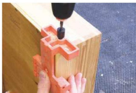
31 Drill stopped holes in the drawer backs for the runner locating pins
