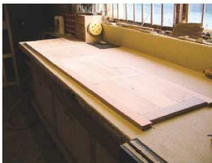
9 Make up the base panel and infill between the rails with tongued-and-grooved boards
