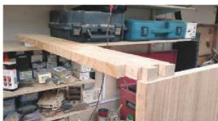
8 Prop the bearer rails in place so you can mark the positions of the dovetails on the sides
