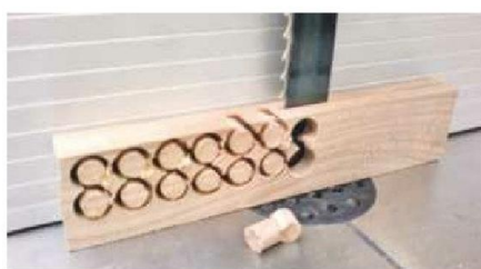
28 Form plugs in a cherry offcut and cut them off on the bandsaw
