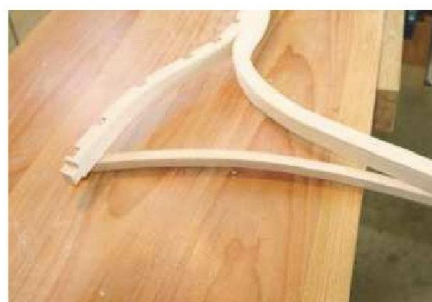
15 Lay the frames over each rib so you can mark the tenon shoulder lines
