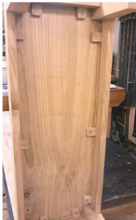
21 Attach the frame to the carcass with a screw through each button
