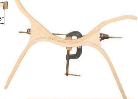
13 Cramp the frames and brackets together so you can measure up for the ribs
