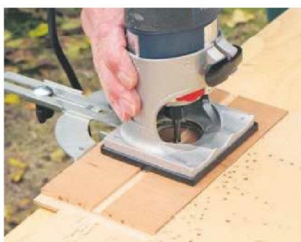
7 Rout through grooves on both end pieces to a depth of 3mm. A simple jig holds these when routing
