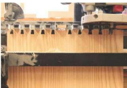
24 Cut the side panel tails first, followed by the end panel pins
