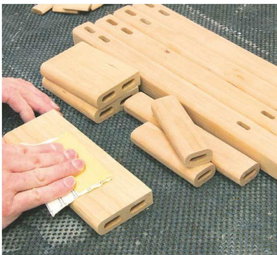
6 Give the legs and rails a thorough sanding before you start the assembly
