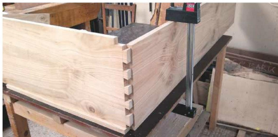
7 Put a 20mm thick shim below the base as you mark the tails on the cabinet sides
