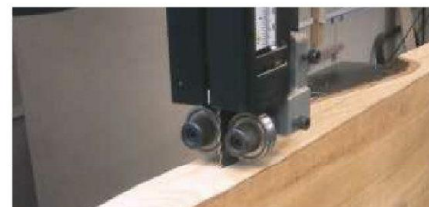
3 Rip each board in half down the middle on the bandsaw...
