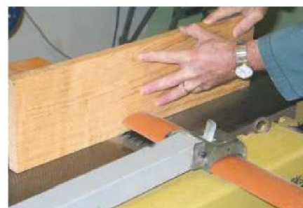
4 Square the edges carefully in preparation for making the L-shaped legs
