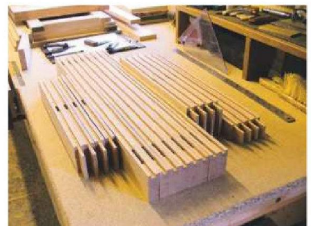
6 Do a head count of the door frame components to check none is missing
