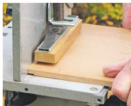
3 Mark out ends of front and back panels. Using a router table, form rebates to half depth of timber
