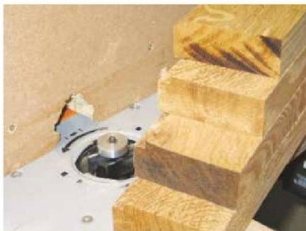
13 Cut the top frame components to length and form a rebate in one edge on the router table
