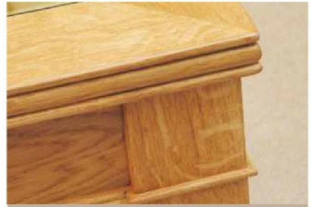
19 Clean up all the edges, apply sealer and wax, and drop the glass into place
