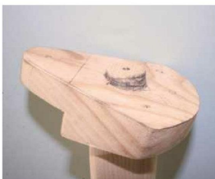
11 Test-fit the legs in the sockets; then select and label the pairs with the best fit
