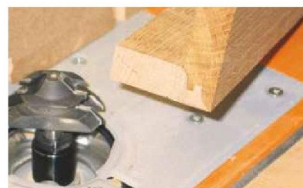
5 I planned to use this cunuing router cutter, called a mitre lock jointer, to assemble the legs
