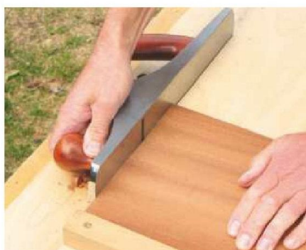
2 Using a shooting board, plane bottom edge of all four panels, plus divider. Trim ends square
