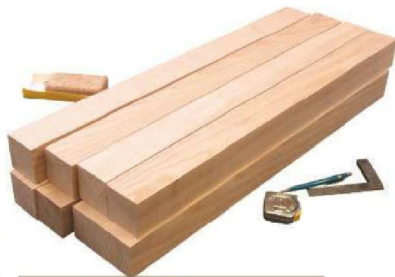
3 Plane each blank flat, square an edge, thickness it and cut it to length
