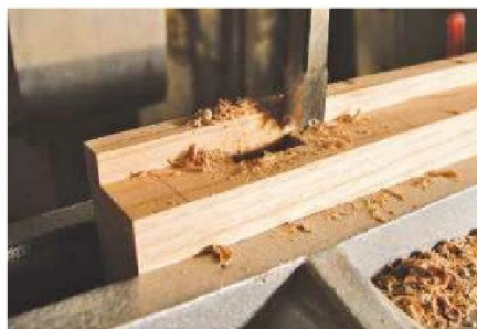
12 Cut the mortise in each door stile tight against the shoulder of the rebate
