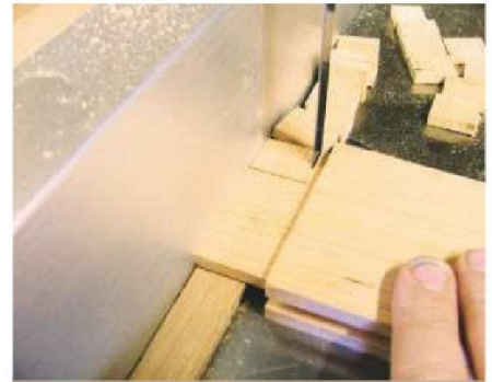
3 Use the bandsaw next to cut down the tenons and form square haunches
