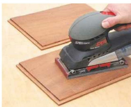
8 Sand inner surfaces with 180 grit abrasive or finer before assembling the box
