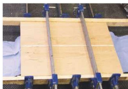
11 Glue up the top boards and cramp them as shown to ensure that they dry flat
