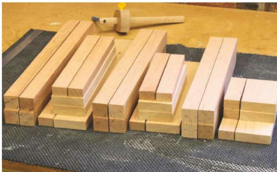
2 Flatten, square and thickness the legs and rails ready for jointing
