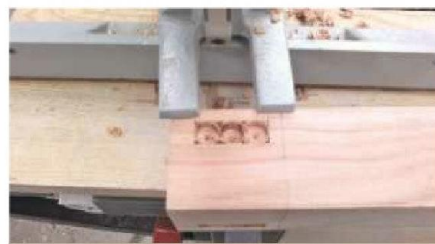
15 Cut the mortises in the base frame members using a mortising machine or pillar drill
