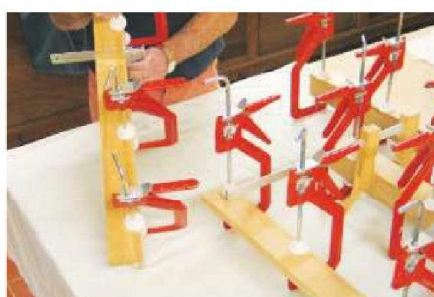
6 Each two-part leg assembly is glued, cramped up and checked for square
