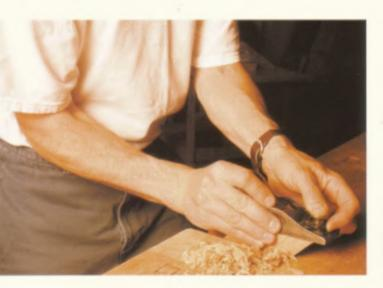
4–21. To brace the plane for a firm stroke, plant your elbow in your hip.
