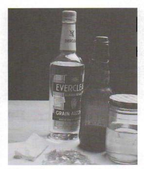
5-42. The products and materials needed for a shellac finish include a pile of blond shellac flakes, a jar of stock-solution shellac, an applicator bottle with diluted shellac, grain alcohol, and an applicator cloth.
