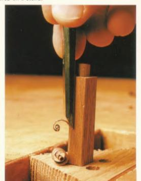
remaining sharp corners of the face that will contact the wedge with a couple of plane strokes. Finally, lightly dome the ends of the tenons, first with slightly arcing strokes of a smooth or mill file, from the perimeter to the center, and then with 220-grit sandpaper (4–64). This helps the cross-pin pop right into place during glue-up and to look nice installed in the cheek.
