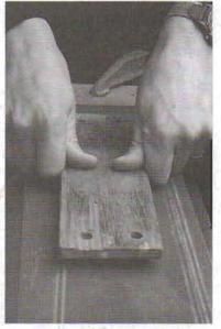
surface of the stone 3-11. A balanced grip for flattenbecomes a uniform ing water stones when dry-sanding.
