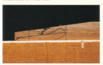
4–92. The layout of a curved wedge on the side of the temporary wedge.
