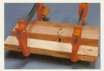
4-66. The alignment stick clamped to the plane bottom.
