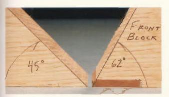
4-117. The front block sawn out, and the insert completed.
