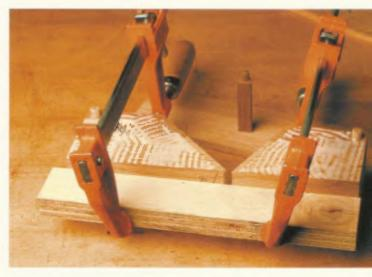
4-69. Gluing one side. Note the cheek with the cross-pin installed.
