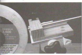
3-5. A diamond dresser mounted in a truing jig. Note the masking tape shim between the lip on the bottom of the jig and the back of the tool rest.
