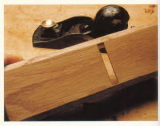
4-111. Chamfers on the bottom.
