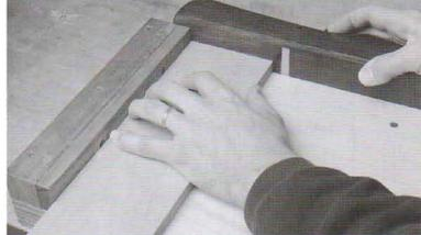
The plane has been set up to produce "square" referenced from the face that is down on the platform. Now check the squareness of the end referenced off the side that was against the stop. If it is off, adjustment is made by removing the stop and tapering it appropriately, or simply by shimming the face of the stop at one end or the other with some strips of masking tape. An alternative, as described above, is to mount an appropriately tapered auxiliary face to the stop.
