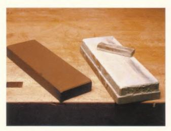
1–4. 800- and 8,000-grit water stones with a nagura, a synthetic stone used to clean the surface of the 8,000-grit stone and create a slurry that speeds sharpening.
