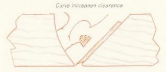
4-5. The curved front block increases finger clearance between it and the cross-pin.
