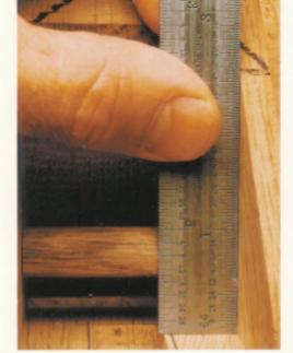
4-71. Measuring the space between the ramp and cross-pin.
