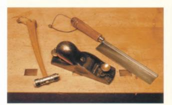
1-1. Hammer, block plane, and fine-tooth saw.
