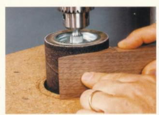
4–93. A sanding drum set up for fairing a wedge curve. Note how the fingers are used to influence sanding.
