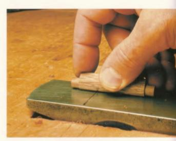
4–63. Shaping the cross-pin by dragging it over a stationary plane.
