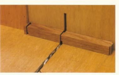
4-55. The setup for the opposite tenon shoulder, with the cuts made.
