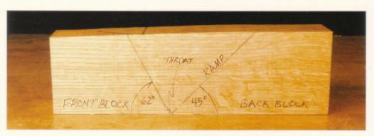
4-2. A plane blank with front-and-back-block layout on the midsection.
