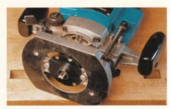
1-5. Router, straight bit, and template bushing.
