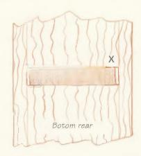
4–89. Sighting the throat opening. The cutting edge was set parallel to the bottom of the plane. The cutting edge is clearly not parallel to the tip of the front block. The right corner of the blade is contacting the front block at the "X."
