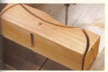
4-105. The shape is sawn out with the band saw.
