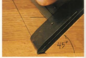
4-38. Locating the face of the cross-pin on the height line 3/16 inch from the chip breaker.
