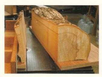
1-31. The band-sawn ash ready for milling off the carrier.
