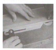
1-17. Capturing the "drift angle" with a bevel gauge.
