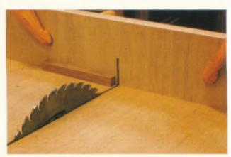
4-53. A crosscut sled with a clamped-on plywood backer. The sled shows a fresh saw kerf that is higher than the cross-pin thickness.
