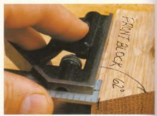
4–28. Marking the tip of the front block  $^{1}/8$  inch up from the bottom.
