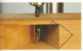
4–41. Drilling the other cheek for the cross-pin through the first hole.
