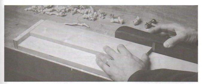
6-5. Using an edge-joining board. The left hand holds the board down and presses it up against the stop. The right hand applies pressure to the front of the plane, keeping its bottom straight on the edge being planed at all times.
