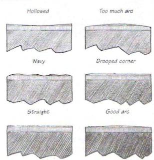
3–42. Assessing the grind of a plane iron. A brief honing polishes the bevel, giving a diagnostic of the shape of the cutting edge.
