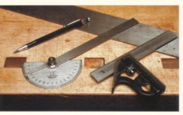
1–3. Pencil, protractor, and 6-inch combination square, resting on an 18-inch straightedge.
