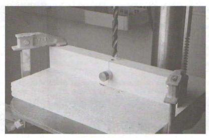
4-78. Drilling a handle hole into the hammer head.
