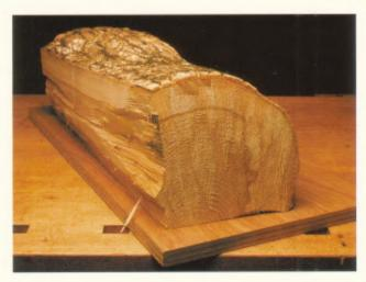
1-30. A firewood chunk screwed to a carrier. Its down side has been flattened on a jointer.
