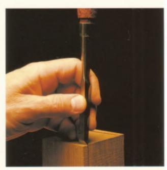
4-36. Separate the cheeks from the blocks by wedging them apart with the tip of a chisel.
