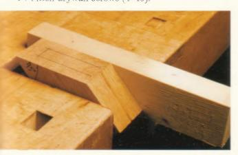
4-45. The scrap board and ramp clamped flush in a vise.
