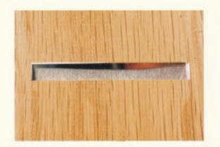
4–88. The cutting edge is still held parallel to the bottom of the plane. The assembly is then sighted toward a bright light. Here, the cutting edge contacts the tip of the front block at the right corner, showing where the front block must be filed to increase the opening and obtain a parallel gap.
