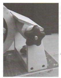
3-3. Side view of a shop-made tool rest.
