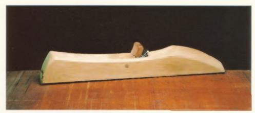
4–128. A jointer plane. It is 17 inches long, and has a  $1^3/4$ -inch-wide iron.
