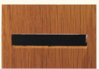
4-98. The completed throat opening is all but undetectable. Sighting it against a bright light reveals a hairthin opening sufficient to allow a thin shaving to pass.
