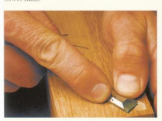
4-35. The thumb guides the chisel to pare dowel ends with power and precision.
