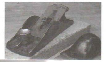
justed. To release the blade, just loosen the cam. Lesser-quality planes rely on a screw working directly on the cap iron to capture the blade. With these, correct pressure must be determined each time the blade is removed and replaced. When the depth of cut is adjusted, the blade should stay clamped. It often takes two or three tries to adjust the blade perfectly; to release and clamp the blade each time the setting is altered would remove all precision from this task.
