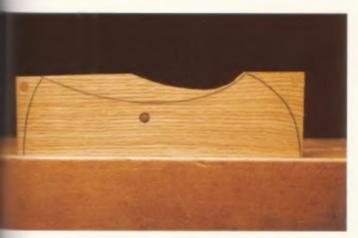
4-104. The shape of the plane is sketched on the side of the blank.
