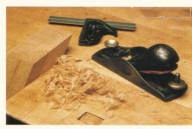
4-20. The front ramp has been smoothed with a minimum of work—just the shavings seen here. For stability it has been clamped low to the bench top.
