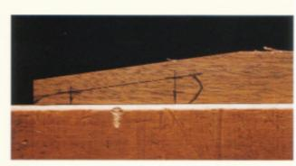
4-91. Lay out the final wedge on the side of the temporary wedge.
