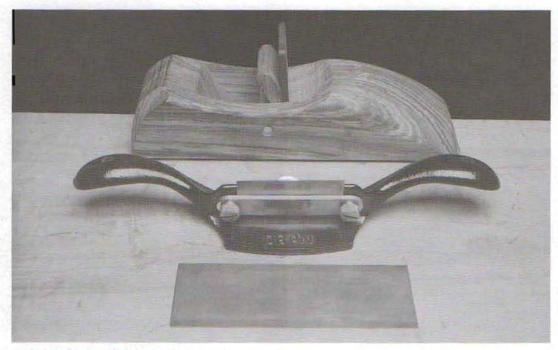
7-1. Basic cabinet scraper (bottom), No. 80 cabinet scraper (middle), and scraper plane (top).
