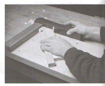
6–10. Shooting an across-the-width miter with a guide screwed to the platform of the end-grain shooting board.
