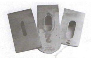
1-33. Various plane irons. Left, specialty iron for wooden planes; middle, Kunz block-plane iron; right, Stanley blockplane iron cut down for wooden planes.
