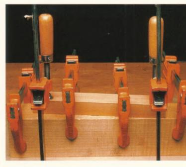
1-32. Gluing set-up for a laminated blank (to avoid gluing it in place, remove the top caul once the other clamps are in place).
