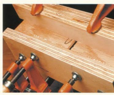
4-70. The glued-up blank with a reasonable amount of glue squeeze-out.
