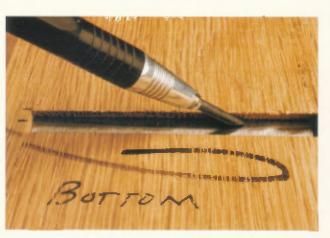
4-83. Marking the front block where the blade contacts it.
