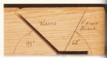
4–115. The saw cuts made on the plane blank.
