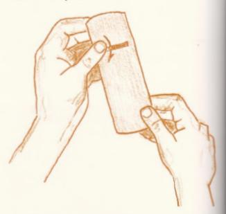
4–8. The thumb is used to feel for the protruding cutting edge.
