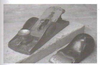
3-1. A look at the plane blade or iron on a disassembled plane.
