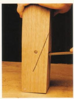
4–90. Filing the tip of the front block to widen the throat opening. The file tip is canted or angled slightly toward the front of the plane.
