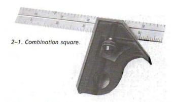
The shavings made with wooden planes on a workaday basis typically range from .001 to .004 inch thick. If the square is off to that degree, or your technique obscures a proper reading, chances are the capabilities of the planes won't be fully utilized. Machinist-grade tools from reputable manufacturers are undoubtedly ready to use off the shelf. Inexpensive hardware-store-variety or flea-market squares usually need work.
