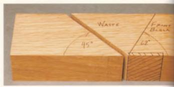
4–114. The insert layout on a plane blank.
