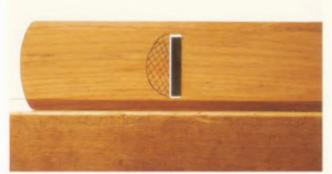
4–113. The cross-hatched area experiences the most friction and wear. Note the relatively wide throat opening.
