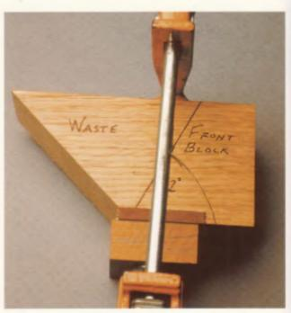
4–116. Gluing the insert. The caul spreads pressure; angling the clamp presses the insert to the front corner of its recess.
