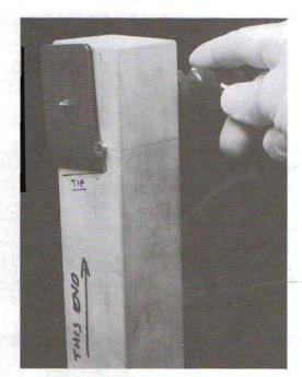
1-43. The chip-breaker tapping jig in use.
