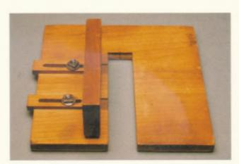
4-48. A ramp-slotting template with an adjustable fence, which also provides a means of clamping the template to the ramp.
