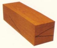
1–24. The sideways "V" keys the plane blank for easy reassembly after resawing.
