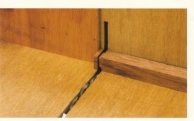
4-54. A close-up that shows the plywood saw kerf aligned with the mark for the tenon shoulder, the stop in place, and the cuts made.
