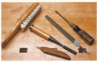
1–2. Shown here are a file card, knife, <sup>1</sup>/2-inch chisel, smooth file, and screwdriver.
