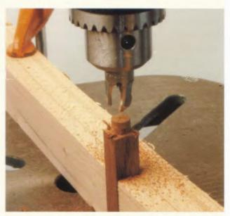
4-59. Drilling a tenon with a plug cutter.
