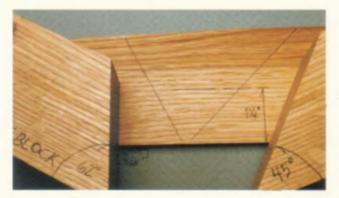
4-37. Lines showing margin of front and back ramps (the outer extent of the sloped portion of the front and back blocks) and cross-pin height.
