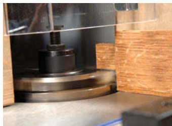
Usinage par-dessous.
